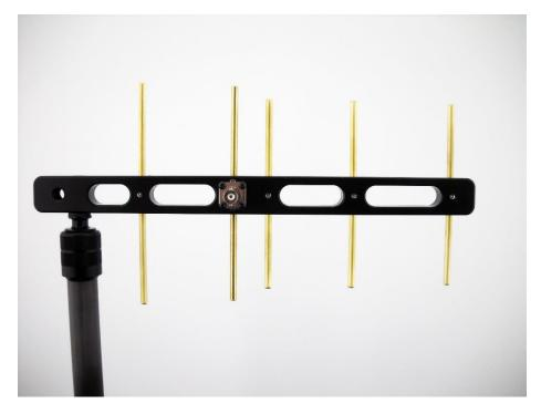
This Photo shows Vertical Polarization of the antenna.
