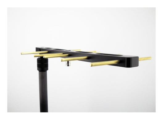
This photo shows Horizontal Polarization of the antenna.
